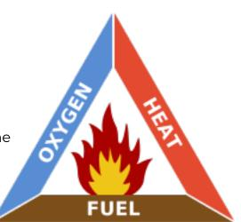
the water to remove the heat from the triangle, whereas a CO2 extinguisher removes the oxygen. A foam extinguisher aims to remove both, with the foam acting as a cooling agent but also a barrier to prevent further oxygen from reaching the fuel source.
